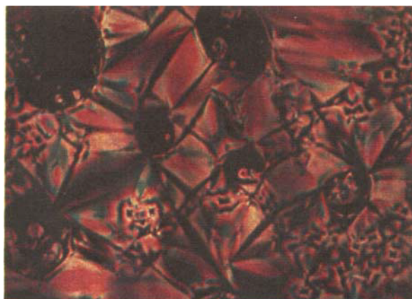
Figure 1. A focal conic texture of CE under crossed nicols. Thickness: 25\mu \cdot 100\times .
